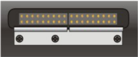
Figure 1-5 Scanner / Audio / Battery Ports – Connector 1 and 2
