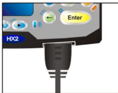
Figure 3-45 Connect ActiveSync Cable to HX2 Cradle Connector
